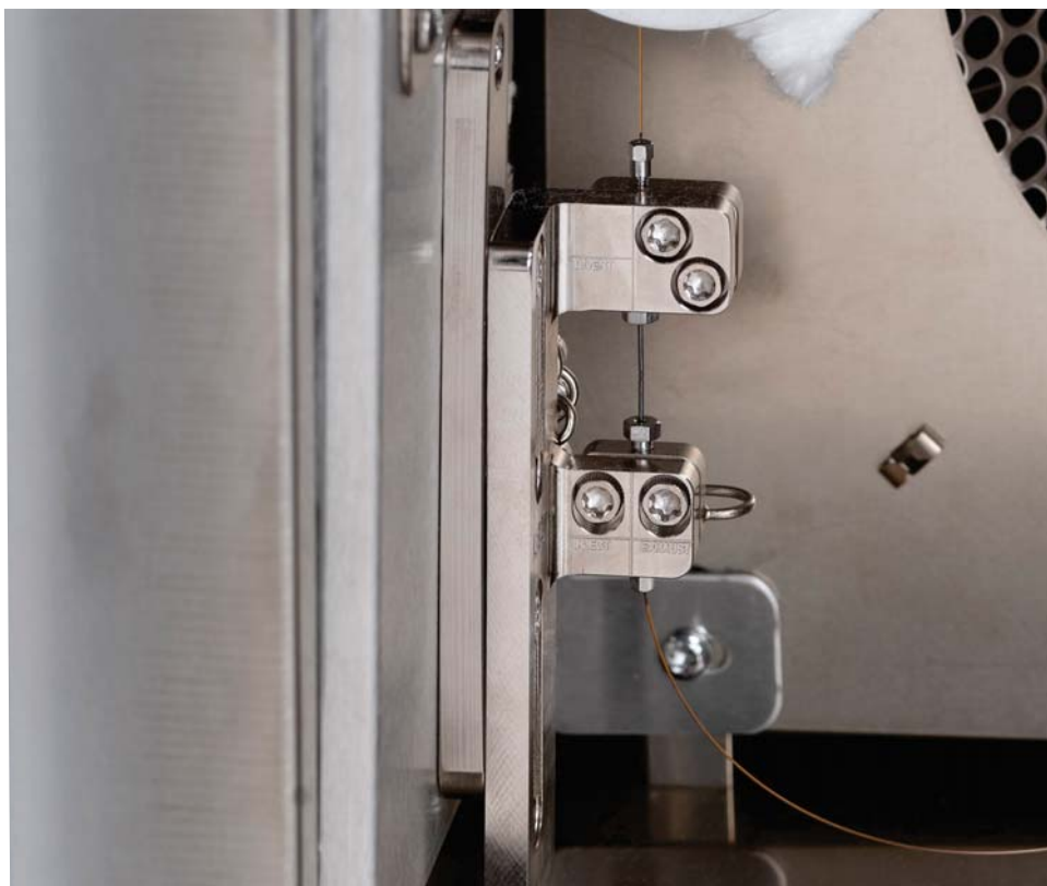
Figure 2. The FLUX flow modulator is pictured right. The tee is mounted to the top portion of the modulator bracket; the cross is mounted to the bottom portion. The cross and tee are connected by a crimped tube which is used to position columns 1 and 2.
