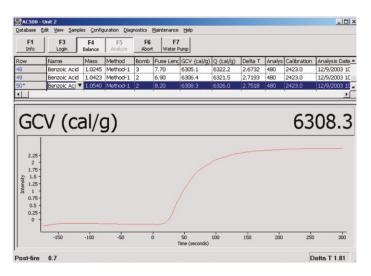
LECO's AC500 software seamlessly manages data, report generation, LIMS compatibility, and can control up to four separate calorimeters through a single PC.
