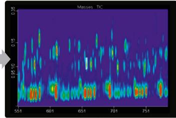
difference in data collected using one-dimensional (left) and two-dimensional chromatography (right).
