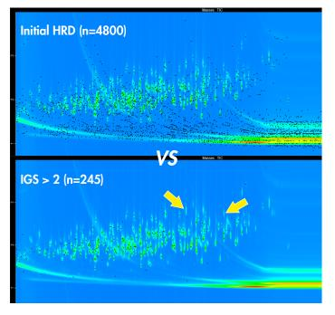
Here is an example of the unfiltered deconvolution results from a GC×GC-TOFMS analysis of a sample from the EPA's ENTACT project:
