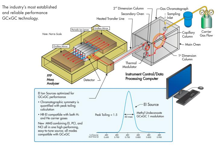
Capable of up to 50,000 mass resolution and acquisition rates up to 200 spectra/second.
