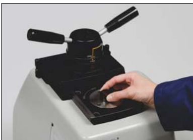
Back-and-forth slide and flip motion mold enclosure provides easy access to mounts
