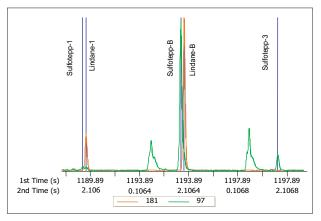
Figure 3. Figure 3 shows that the integration of each slice equals the total area observed in the 3D view. The linear chromatogram shows the uncombined peaks and labelled peak markers for Sulfotepp and Lindane over the GCxGC modulations of 4 seconds each from 1189 to 1197 seconds in the first dimension.
