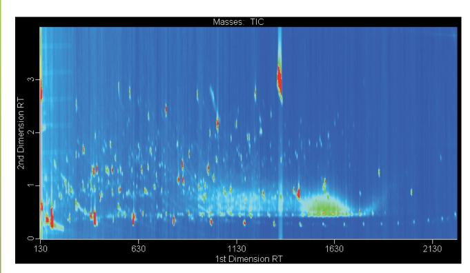
Figure 1. GCxGC-TOFMS contour plot of brewed green tea with OCP/OPP pesticides showing over 1200 peaks at a S/N ratio of 100.
