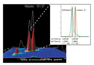
Figure 4. The GCxGC-TOFMS surface plot of 500 ppt spiked standards of Sulfotepp (mass=97) and Lindane (mass=181) illustrates the resolution in the second dimension of the chromatographic plane. The inset is the zoomed in linear chromatogram of the modulated slice for the base peaks of Sulfotepp and Lindane. These two pesticides coelute at 1193 seconds in the 1st dimension. However Sulfotepp and Lindane are separated by 132 milliseconds in the second dimension.
