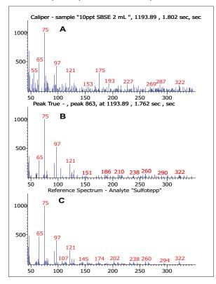
Figure 5. Shown in succession is the Caliper–Total Ion Mass Spectrum (A), The Peak True–Deconvoluted Mass Spectrum (B), and the Reference-Mass Spectrum (C) for 10 ppt of Sulfotepp spiked in brewed green tea.
