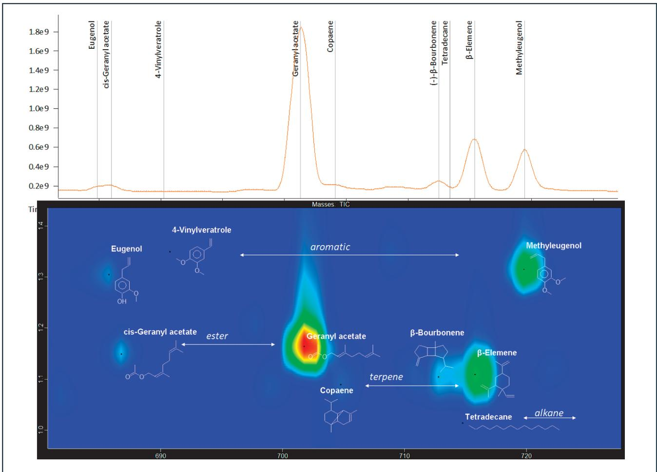
**Figure 2. GCxGC separates the samples based on two mechanisms, providing insight to chemical structure based on retention in the second dimension.**
