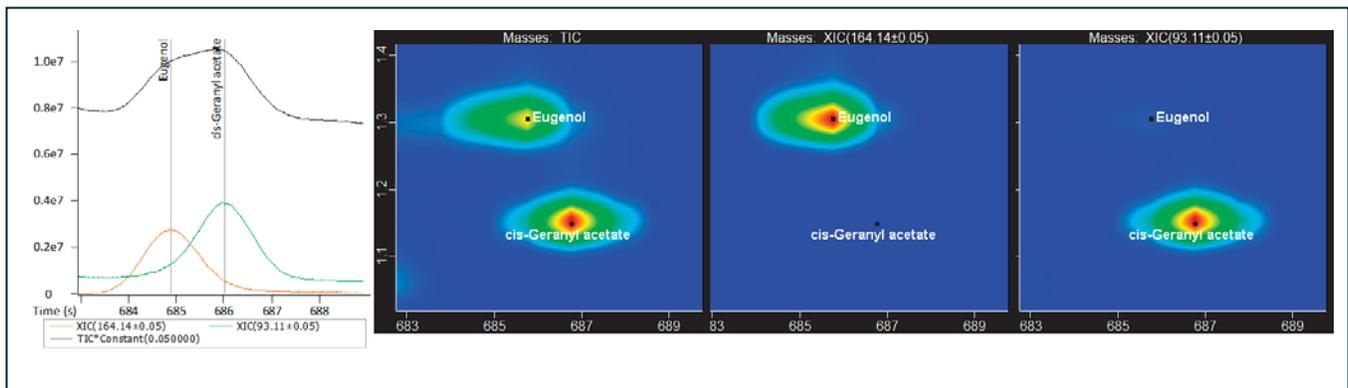
**Figure 3. TIC and XIC traces associated with the first two peaks in Figures 2. These analytes coelute with GC, but are separated in the second dimension with GCxGC.**
