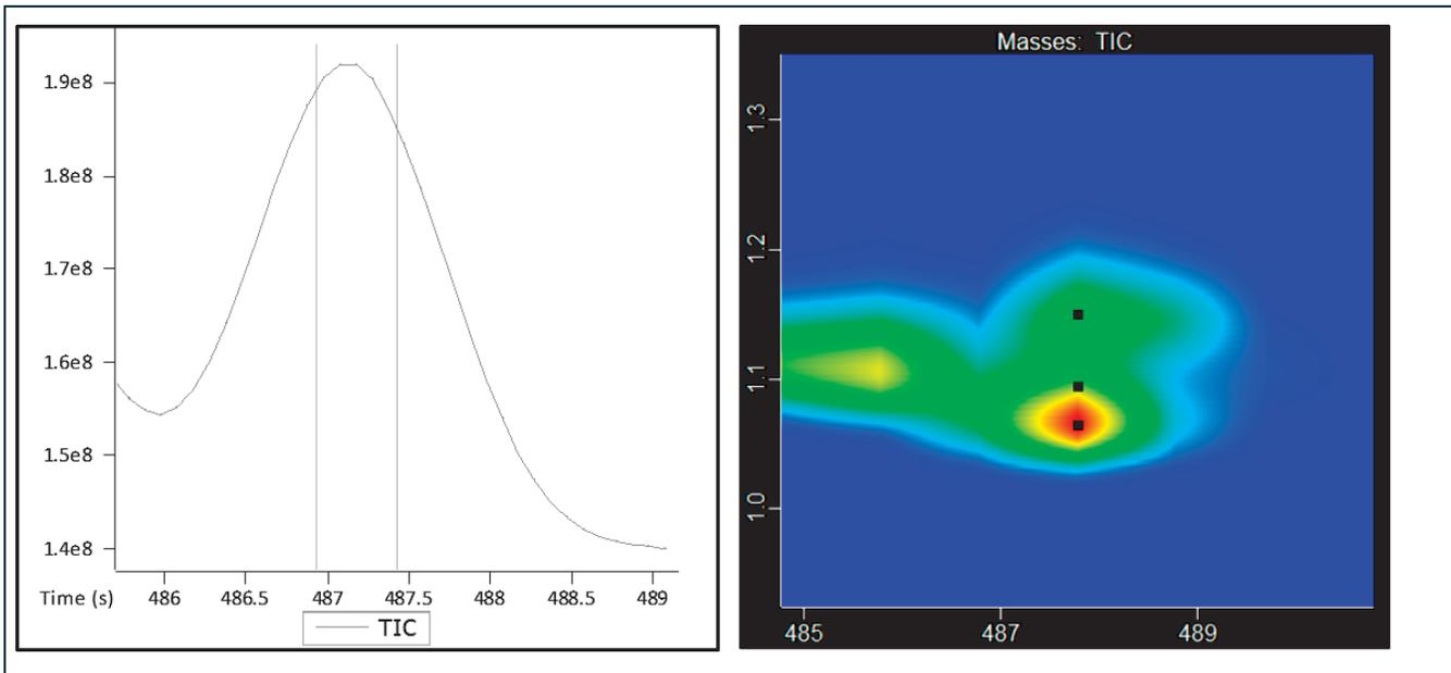
**Figure 4. GCxGC can chromatographically separate some analytes that coelutes in the first dimension, increasing the peak capacity in instances of perfect coelution. What was determined to be two peaks in the GC data, was found to be three in the GCxGC data.**
