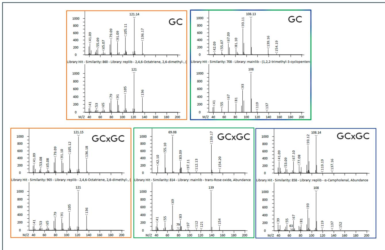
**Figure 5. Spectral information for analytes that separated with GC and GCxGC. With GC, two of the three peaks perfectly coelute and are combined in a single peak marker and spectrum.**
