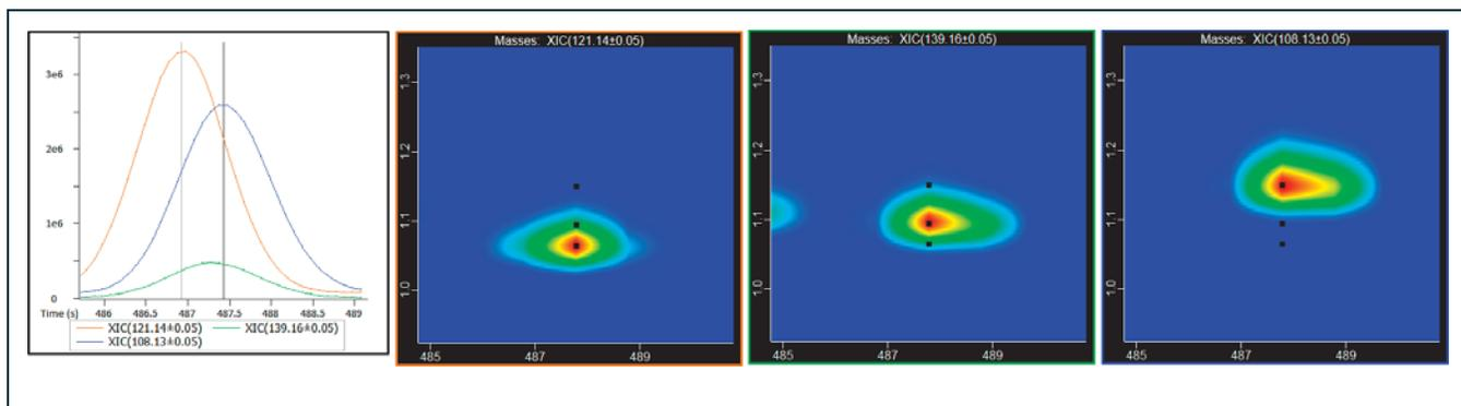
**Figure 6. XIC traces associated with the peaks in Figures 4 and 5. Two of the analytes that perfectly coelute in GC are separated in the second dimension with GCxGC.**
