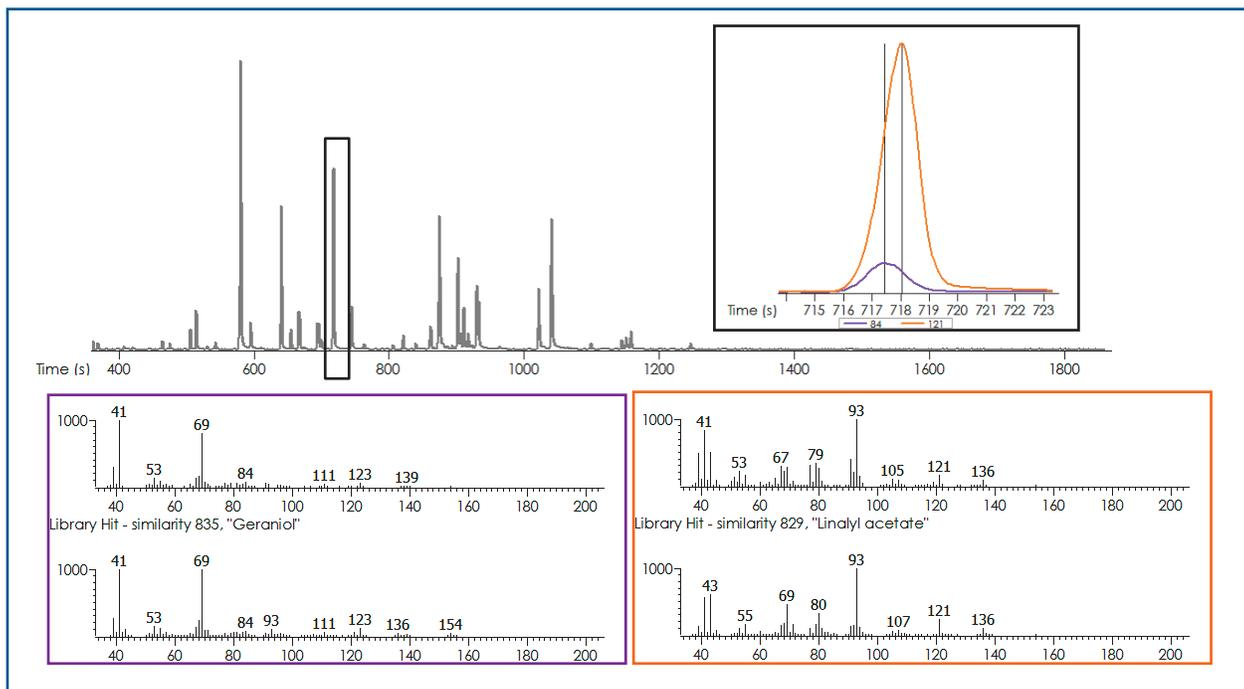
**Figure 3. Geraniol, a target allergen, coelutes with a matrix analyte, tentatively identified as linalyl acetate. ChromaTOF's deconvolution capabilities mathematically separates this coelution and provides pure spectra and pure peak profiles for each analyte. There are several shared  $m/z$  between these analytes.**
