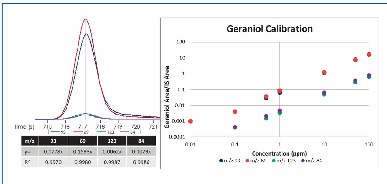
**Figure 2. Geraniol is chromatographically isolated in the allergen standard and several m/z are unique and appropriate for determining calibration equations. m/z 93, 69, 123, and 84 are all free from interferences and provide reliable calibration information. SIM methods often suggest m/z 93, 69, and 123 for this analyte.**
